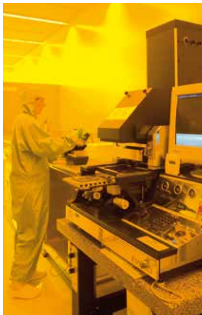
Photolithography: generating the structure on the substrate
