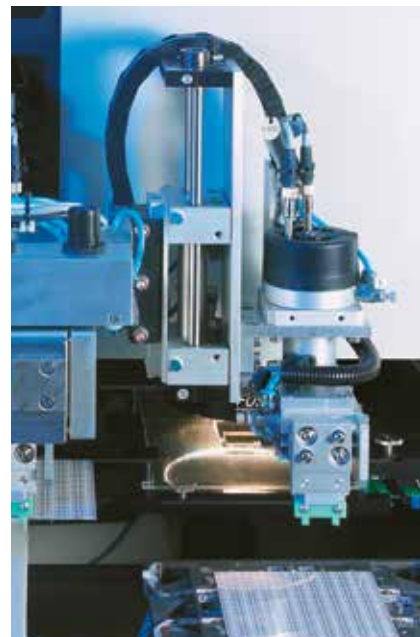
Laser calibration of platinum chip temperature sensors
