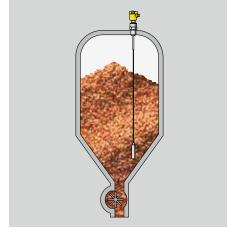
Level measurement in a grain silo
