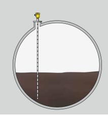
Level measurement in a gas tank (LPG)
