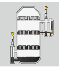
Measurement in a distillation column
