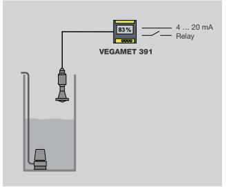
VEGAPULS WL 61 can be integrated into an existing control system in different ways depending on its configuration. Both analogue and digital sensor versions are available.
