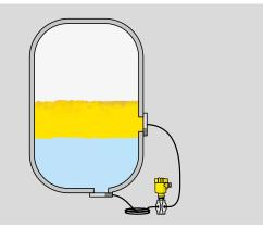
Chemical seal both side assembly (CSB) • For density or interface measurement
