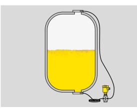
Chemical seal both side assembly (CSB)For level measurement in vessels with head pressure
